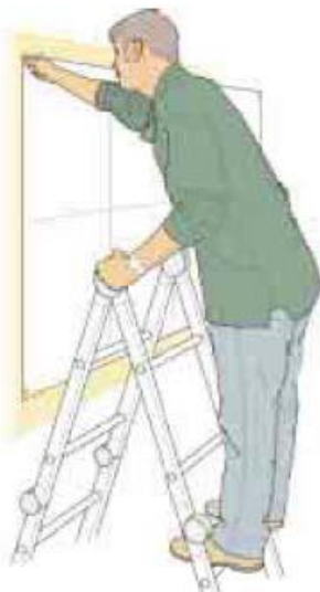
Correct – two clear rungs. Don't Work any higher up this type of stepladder.
