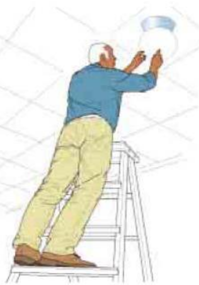
Correct – 3 clear rungs, do not work any higher on this type of stepladder
